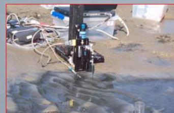
Our sulfate micro electrodes exhibit a Nernstian response to sulfate in the concentration range from  $10^{-6}$  to  $10^{-2}$  M and work well in fresh waters.
