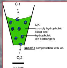
We have adapted a potentiometric sulfate microsensor for *in-situ* measurements that has a membrane containing an ionophore with a high selectivity for sulfate.
