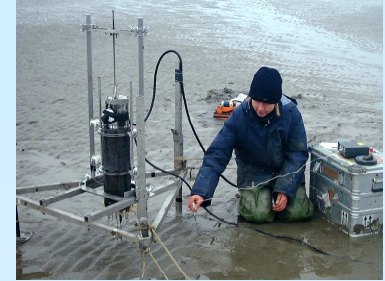
Fig. 1. Lander used for in-situ microsensors measurements.
