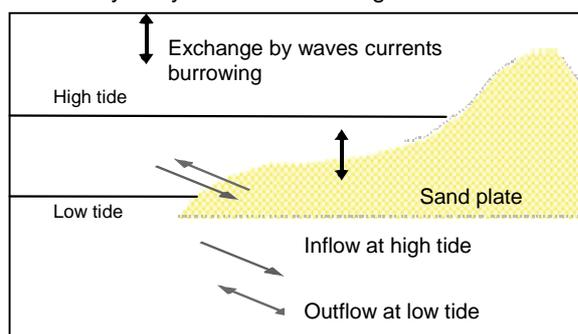
Fig. 1. Sketch of the main advection phenomena on intertidal sand plates.
