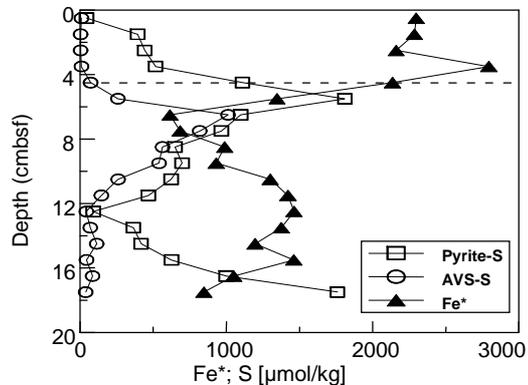
Fig. 5. Downcore variations of sedimentary sulfur species (AVS and pyrite sulfur) and reactive iron (Fe\*) at a sandy site in fall. Dashed line marks the supposed maximum oxygen penetration or resuspension depth.
