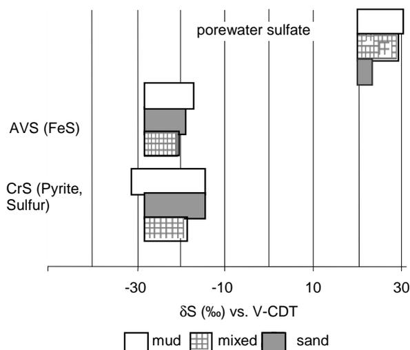
Fig. 8. Stable sulfur isotope discrimination between sulfate and the CRS and AVS fractions.
