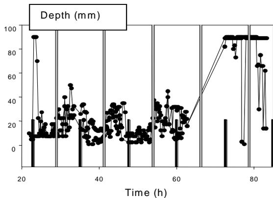
Fig. 3. Penetration depth (in mm) of oxygen measured, over a period of several days with microsensors mounted on a lander. The interruptions of the measurements were caused by broken sensors.
