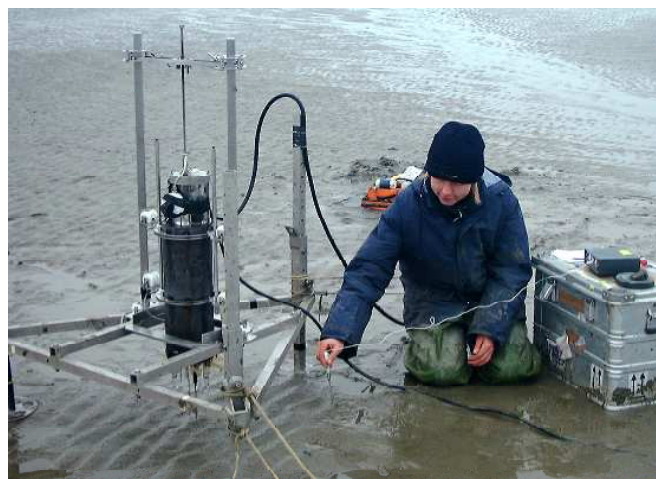
Fig. 2. Lander used for in-situ microsensor measurements.
